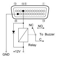
NC: Normally Closed Contact NO: Normally Open Contact
