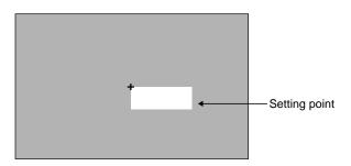
2. Move the "+" mark to the desired area, and then press the CAM (SET) key. Setting point 2 is determined and the "+" mark will disappear. Then, the mark will appear again at the center of the monitor. The square, covered with Setting point 1 and 2, is showing the motion-detection area.
