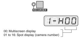
3. To exit from the recorder mode, select the camera. (Refer to p. 91 Camera Selection.) The indicator beside the button will go out. The monitor number and camera number will appear on the LED display again.
