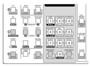
To end the setting and return to the normal view, press the SETUP button while holding down the SHIFT button when SETUP MENU is displayed. The system controller's SETUP indicator will go out.
