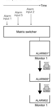
**Note:** When more than one alarm is input and they are associated with the same monitor, they will be reset one by one.
