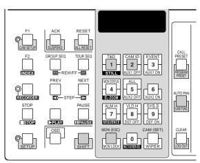
Press the button 1 to change the image from the color mode to the black and white mode on the active monitor.
