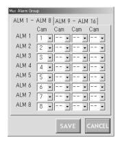
This is a submenu of the Multiplexer window. In this window, up to 4 cameras are given recording priority for each alarm input.
