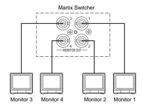
Monitor 1 to 4. When you control the monitors from a PSD ata controller, the connectors MONITOR OUT are associated to Unit 1 to 4.
