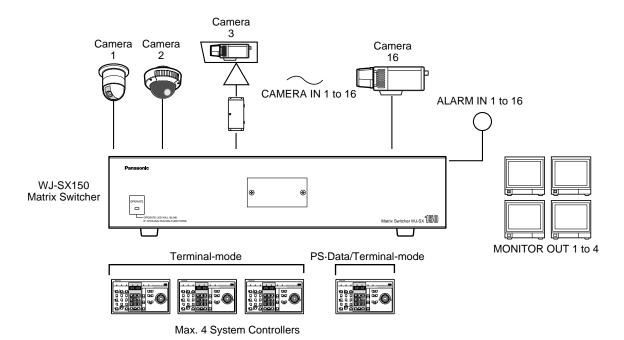
**Note:** Before connecting a terminal-mode system controller to the DATA 4 port, configure the system through SETUP MENU or WJ-SX150 Administrator Console.
