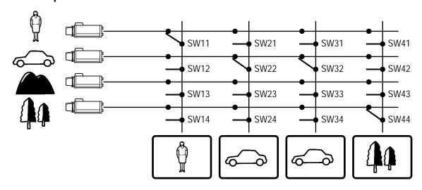
All matrix switchers, no matter how complicated and sophisticated they may be, depend on crosspoint switches to perform the basic operations of the switcher. The crosspoint switches from a rectangular array of rows and columns in which any row may be connected to any column.
